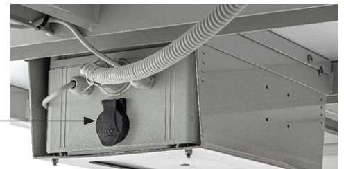
Charging connector on the shower trolley
