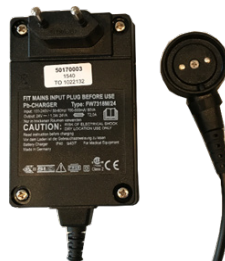
Charging connector on battery charger
